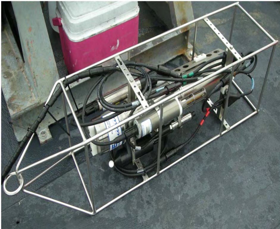
SBE-19 Plus Water Quality Instrument
